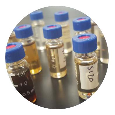
pump suction will provide the lowest temperature/ lowest pressure sample point in the system. Samples should not be taken from the expansion tank or any dead legs — the sample may be easier to handle but will not be representative of what is actually circulating.
